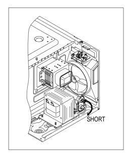
**CAUTION**: Service personnel should remove their watches whenever working close to or replacing the magnetron.
